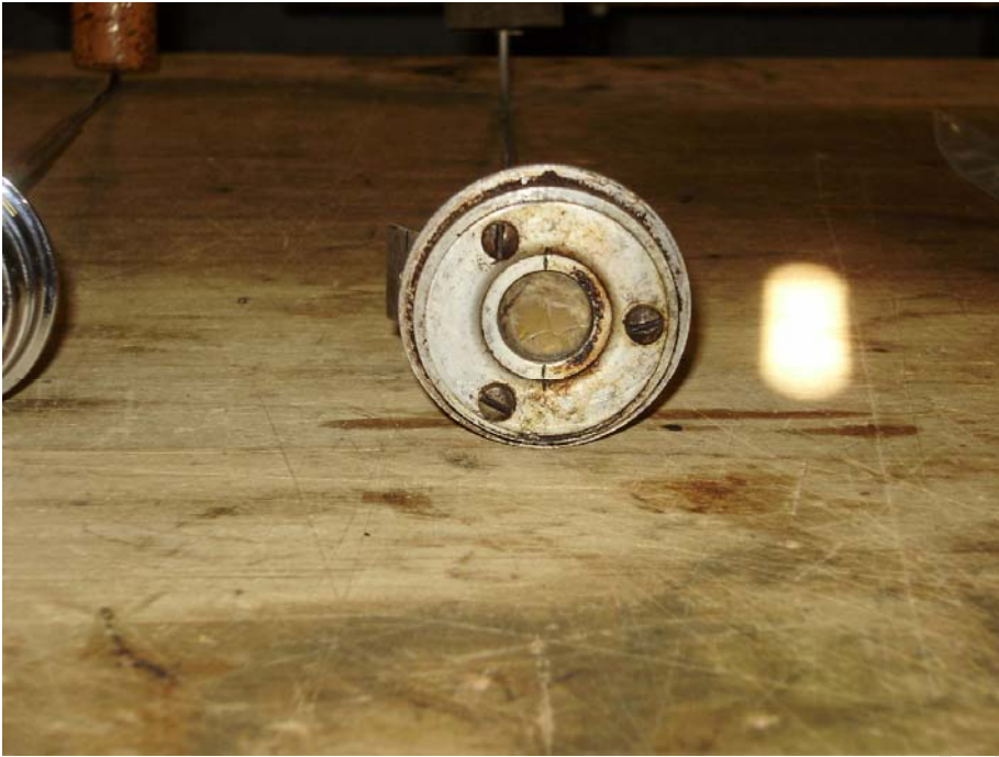
PICTURE IS A TYPICAL HARDING GAUGE- NOTE THE STAINED AND CHIPPED PLASTIC FACEPLATE
