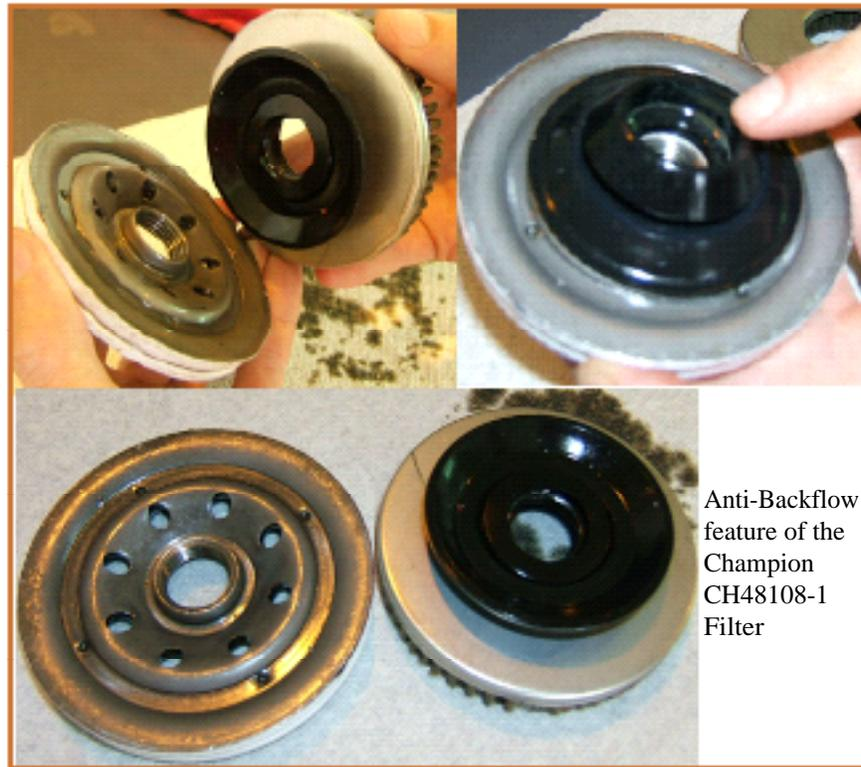
Per Alex of Champion, those filters manufactured December of '04 and after will be the newer type; the older filters have only four inlet holes whereas the newer have the eight holes shown here, and the latest also have the more limber anti-flowback for better sealing, .
