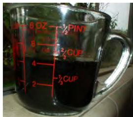
The actual amount of oil that comes out of the screen chamber is shown in the measuring cup, about two thirds of a cup. If you leave that amount of dirty oil in place, along with the oil captivated in the galleries (you cannot drain them), you immediately get a contamination of the clean new oil with the chemically active old oil. Your choice.
