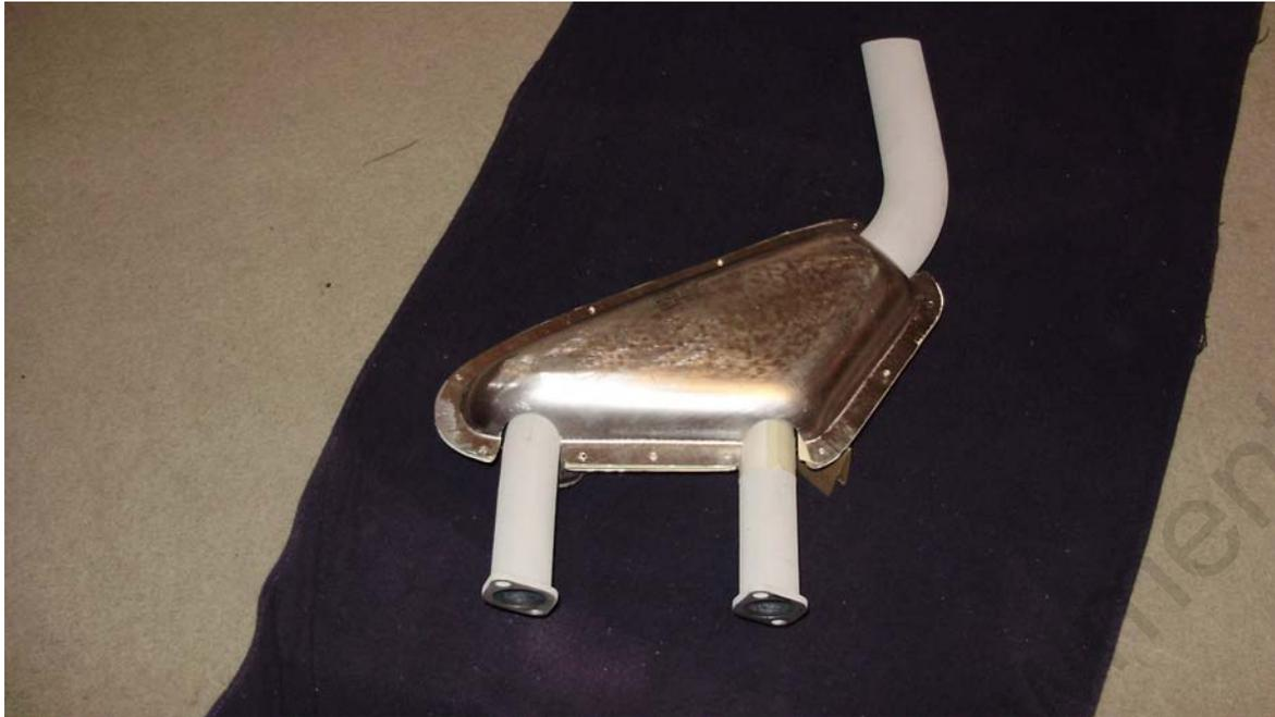
Again, it is usually necessary to relieve the muff where it meets the exhaust pipes so that there is about .030" to .100" clearance at the exhaust tubes and the muff to allow some hot air to escape while providing some cooling air to the aluminum muff to keep it from melting on the hot stack. The clearance should look like this:
