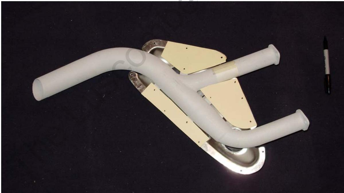
With the baffles properly mounted to the stack tabs, the clamshell muff parts are then mounted to the baffles around the perimeter flange, using screws on about a 2 to 3" center:
