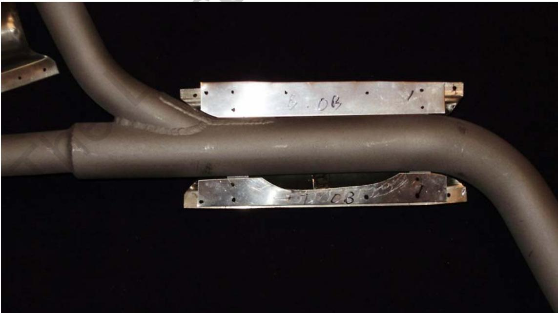
In fitting this system up, there will be some anomalies between stacks and stack manufacturers. It is usually necessary to relieve the muff where it meets the exhaust
